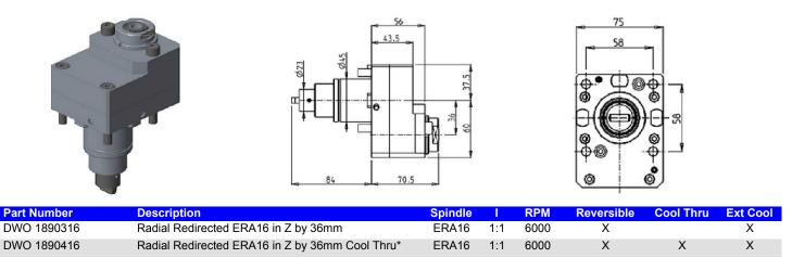
\* Coolant Thru tools are designed for 1000 psi. They require 5 Micron Filtration and CANNOT be run dry.
