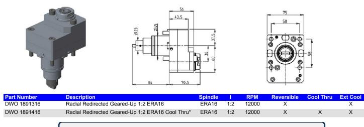
\* Coolant Thru tools are designed for 1000 psi. They require 5 Micron Filtration and CANNOT be run dry.
